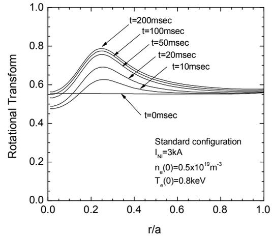
Fig.2. Rotational transform profile EC current density profiles calculated by TRAVIS code
