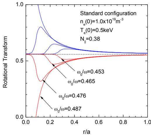
Fig.1 Rotational transform profiles modified by ECCD
