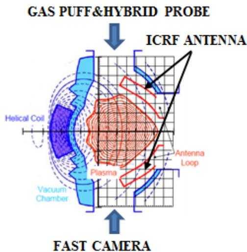
Fig. 2 Crosssection of #14.5 port section where ICRF antenna is installed. The fast camera is set at the bottom port and the gas-puff and the hybrid probe are installed at the top port. The vacuum flux surfaces of the standard field configuration are also illustrated.
