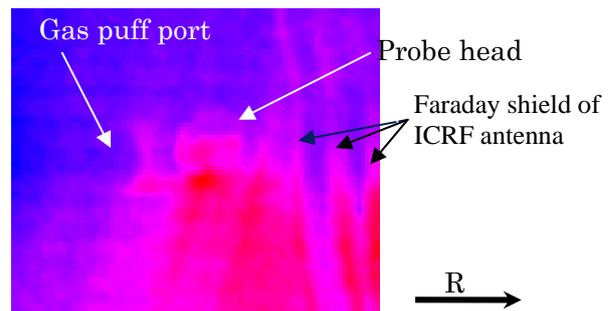
Fig.3 Snapshot image of an NBI plasma with SMBI (#11.5) and GPI (#14.5) at #14.5
