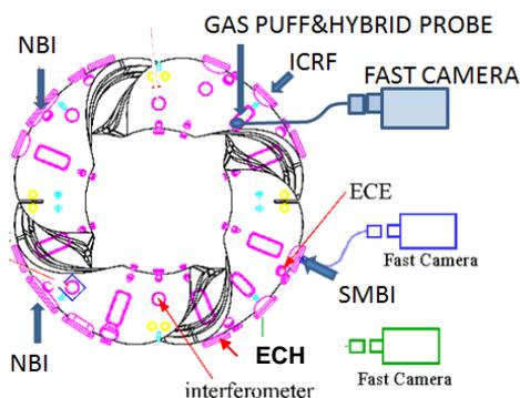
Fig.1 Top view of Heliotron J. The locations of fast cameras, the gas puff for GPI and the hybrid probe are illustrated.
