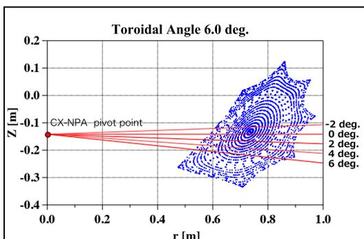
Fig.2 Line of sight of the CX-NPA in the plasma cross section at  $6.0^\circ$  in toroidal angle.
