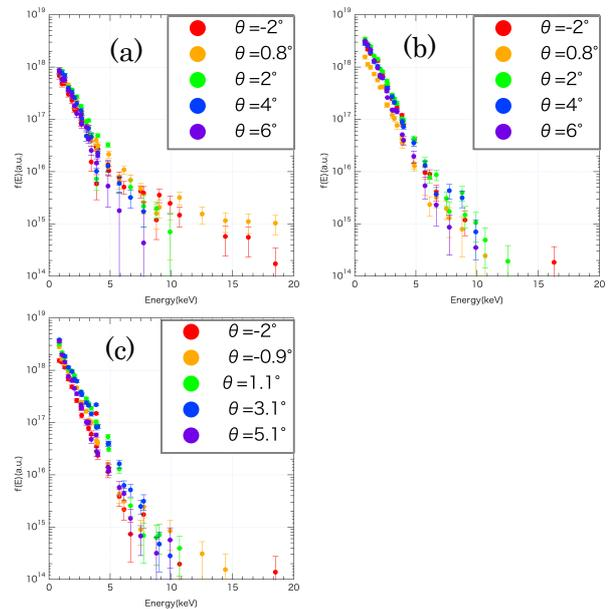
Fig.3 Energy spectra measured at the toroidal angle  $6^\circ$  for (a)high bumpiness, (b)medium bumpiness and (c)low bumpiness
