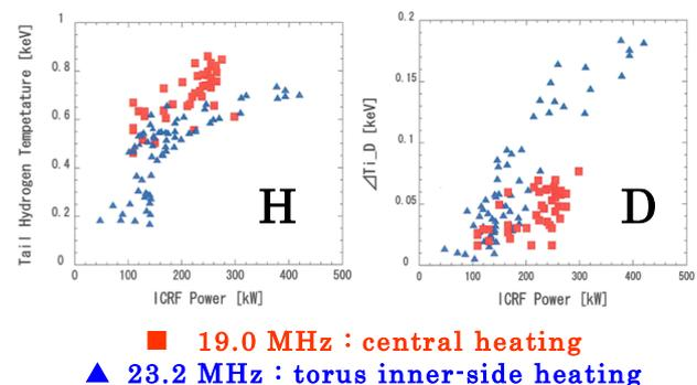
Fig.1 Heating position dependence of the effective temperature in the CX-NPA measurement line of sight is faced to magnetic axis.
