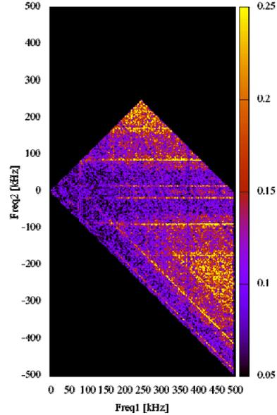
Fig.3 Result of bicoherence analysis for ion saturation current fluctuation measured with #11.5 probe at 4mm inside LCFS.
