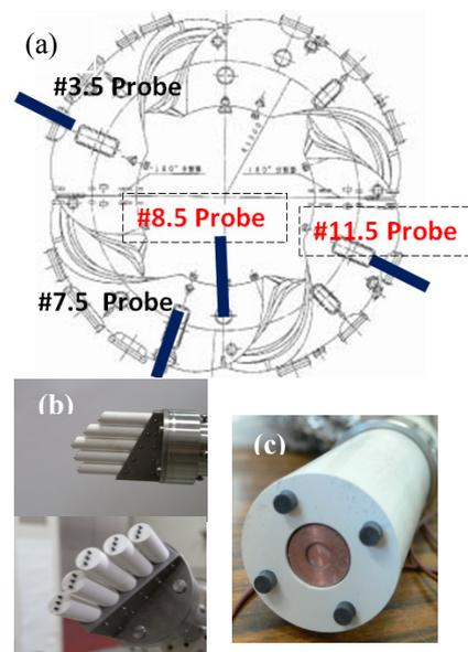
Fig.1 (a)Probe locations in the top view of Heliotron J. (b)Probe heads at #11.5 section and (c) probe head at #8.5 section.
