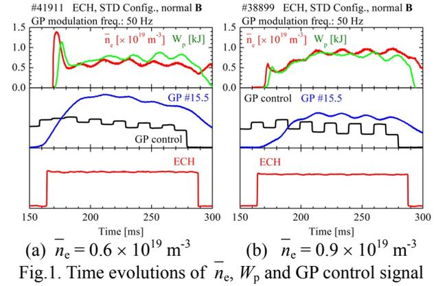
Fig. 1. Time evolutions of  $\bar{n}_e$ ,  $W_p$  and GP control signal
