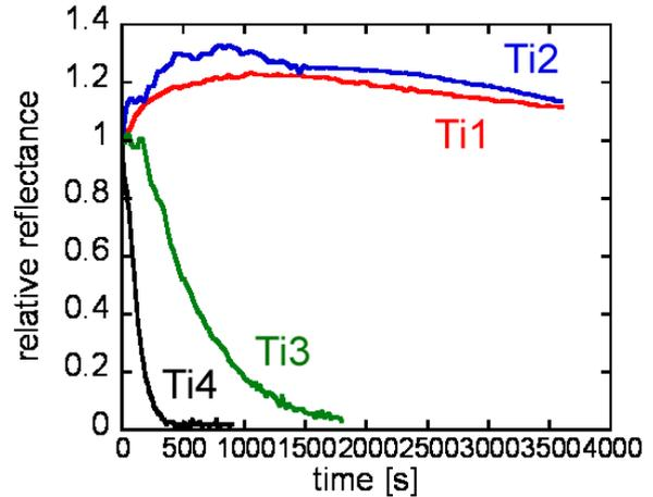
Fig. 2. Measured relative reflectance of titanium under helium plasma exposure; the detail exposure conditions are summarized in Table 1.
