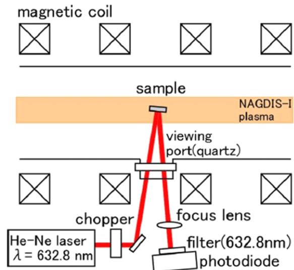
Fig. 1. A schematic of relative reflectance measurement setup
