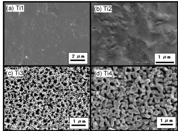
Fig. 3. SEM micrographs of titanium exposed to helium plasma under the conditions shown in Table 1.
