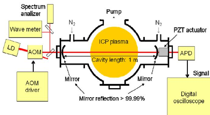
Fig. 1 Experimental setup for cavity ringdown spectroscopy.
