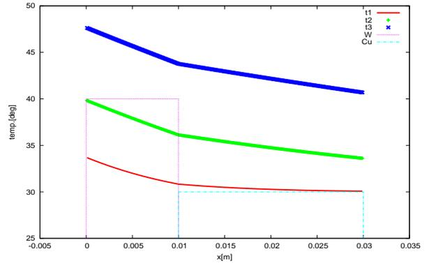
Fig.3: Calculated temperature profile. Initial temperature is assumed to be 30 [deg.], plasma irradiation starts at  $t = t_0 = 10$  [s], and three profiles for  $t - t_0 = 1.0, 10.0,$  and  $50.0$  [s] are plotted.  $L_{ex} = 100L_1$  is assumed.
