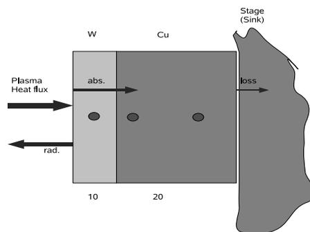
Fig.1: Schematic drawing of composite target. The target consists of Tungsten (1cm thick) and Copper ( 2cm thick ).
