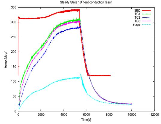
Fig.2: Example of temperature evolution. RF power for plasma production is about 400[W]. Discharge duration is 90 [mini.].
