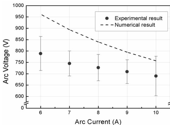
Fig.2. Arc voltage comparison between experimental and numerical results according to arc current.
