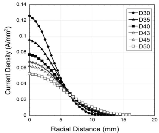
Fig.4. Radial profiles of arc current density on the middle of the arc channel ( $z=200$ ) for different tube diameters.
