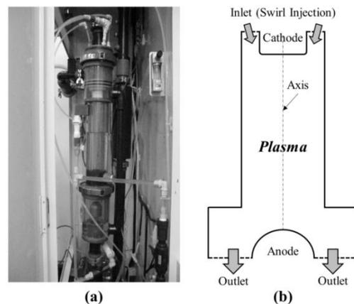
Fig.1. (a) photograph of the long DC arc system, and (b) computational domain on the plasma region.
