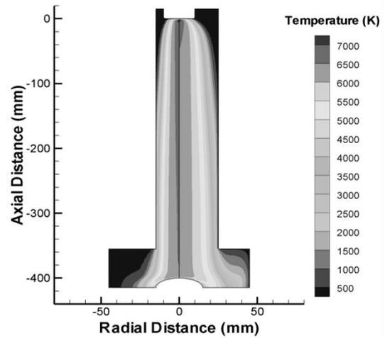
Fig.3. Comparison of temperature distributions between  $D=30$  and  $50$  at operating conditions of  $10$  A and  $30$  lpm.
