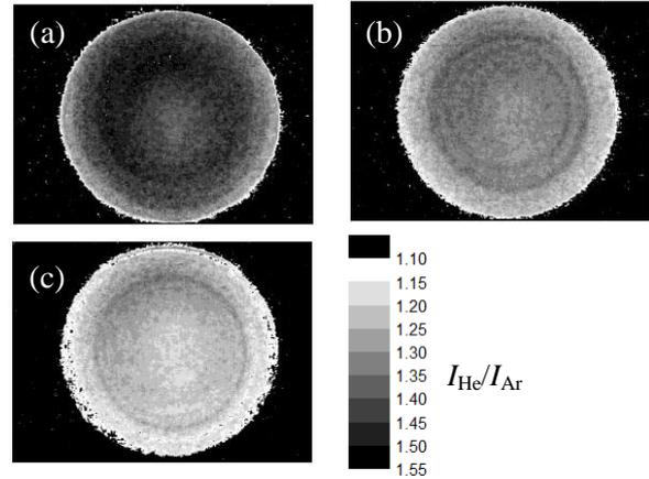
Fig. 4. Spatial profile of  $I_{\text{He}}/I_{\text{Ar}}$  in He/Ar/HBr plasma at total pressures of (a) 30 mTorr, (b) 50 mTorr, and (c) 70 mTorr.
