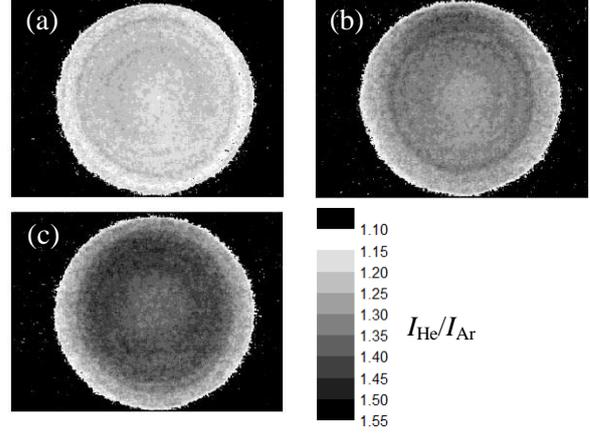
Fig. 3. Spatial profile of  $I_{\text{He}}/I_{\text{Ar}}$  in He/Ar/HBr plasma at HBr flow rates of (a) 6 sccm, (b) 12 sccm, and (c) 18 sccm.
