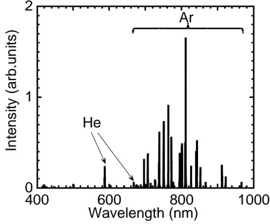
Fig. 2. Typical emission spectrum of Ar/He ICP plasma.
