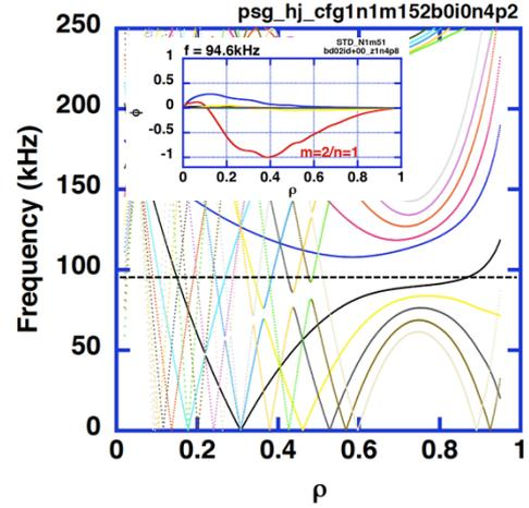
Fig.1. Example of shear Alfvén spectra including continua and eignfunction for  $N_f=1$  of Heliotron J.
