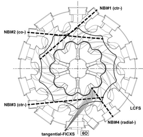
Fig. 1 Hardware apparatus of tangential FICXS diagnostic on the midplane of LHD.
