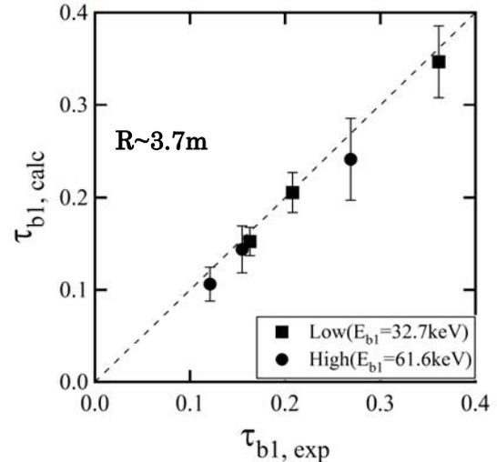
Fig. 2 Comparison between slowing down time obtained by calculation and observed FICX signal.
