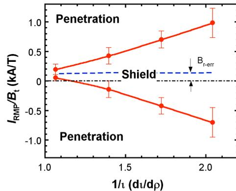
Fig.3 Change of mode penetration as a function of magnetic shear on  $\iota/2\pi=1$  resonance.
