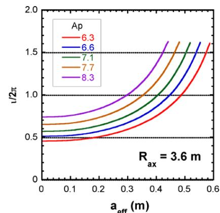
Fig.1 Rotational transform profiles in different  $A_p$  configurations.
