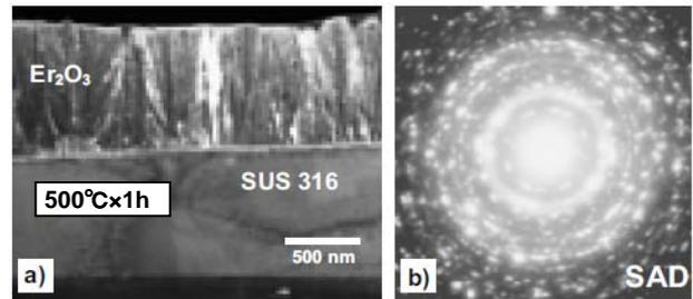
Fig.2. TEM and SAD images of  $\text{Er}_2\text{O}_3$  coating layer via MOCVD process
