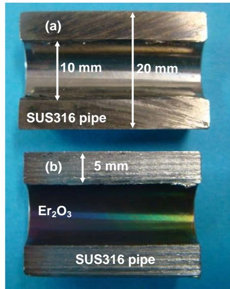
Fig.3. Typical photograph of the interior surface of the SUS pipe before and after MOCVD  $\text{Er}_2\text{O}_3$  coating. (a) Before MOCVD coating, (b) After MOCVD coating
