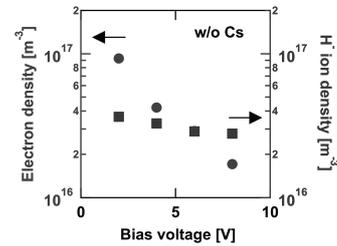
Fig. 4. Dependence of electron density and  $H^-$  ion density on bias voltage.
