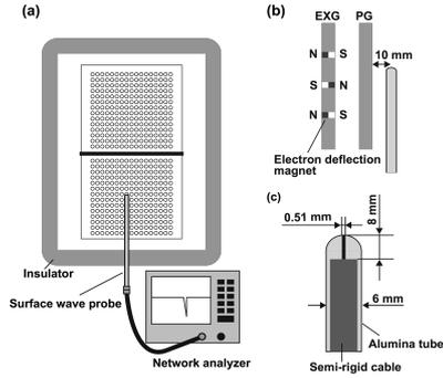
Fig. 1. (a) Schematic illustration of experimental setup, (b) positional relation of SWP with PG, (c) cross-sectional view of SWP.
