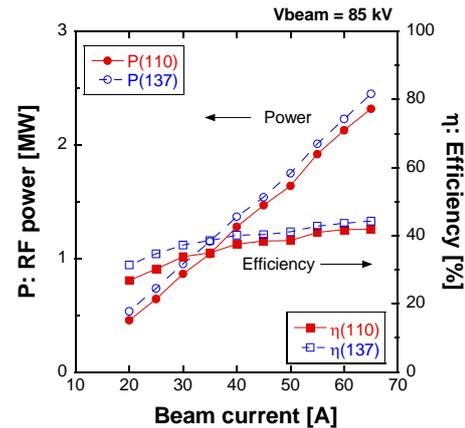
Fig.2. Simulation result of beam current dependence of generated rf power and efficiency of the newly designed gyrotron cavity. The cavity magnetic field was optimized to obtain the highest efficiency with the electron pitch factor and beam voltage of 1.1 and 85 kV, respectively.
