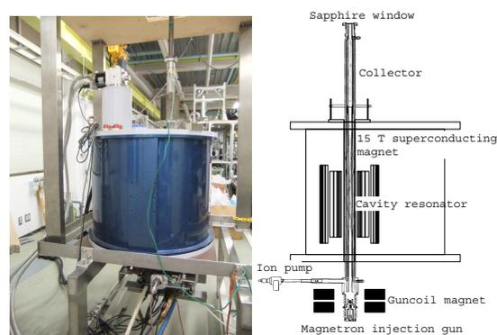
Fig.1 Sealed-off gyrotron (Gyrotron FU CW VIB) and a 15 T superconducting magnet.
