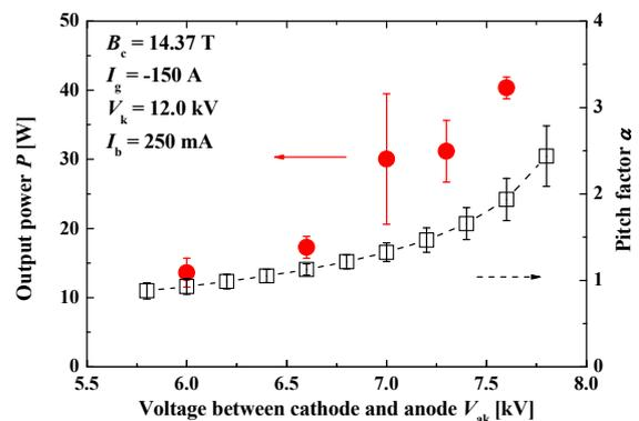
Fig.4 Output power and calculated pitch factor as a function of the voltage between cathode and anode.
