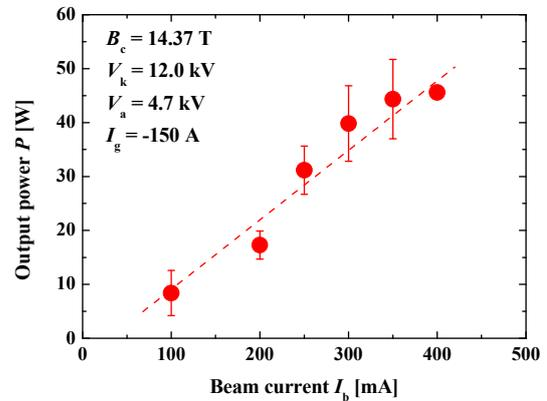
Fig.3 Output power as a function of beam current.
