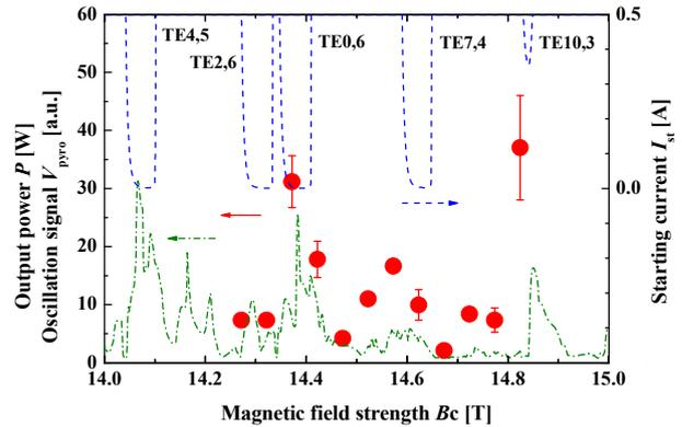
Fig.2 Oscillation signal, output power and calculated stating current as a function of magnetic field strength.
