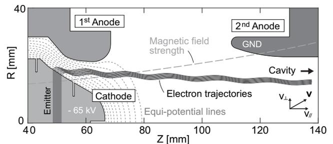
Fig. 1. A schematic diagram of MIG.
