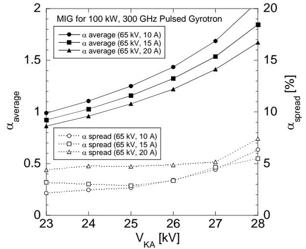
Fig. 3. Calculated pitch-factor  $\alpha$  and  $\alpha$  spread for 65 kV, 10-20 A electron gun.
