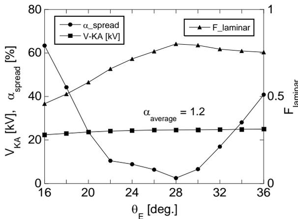
Fig. 2. Variation of the  $V_{KA}$ , the  $\alpha$  spread at the cavity and the degree of the lamination is given as functions of the slant angle  $\theta$ . In the calculations, the averaged value of  $\alpha$  at the cavity is fixed by changing the  $V_{KA}$ .
