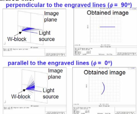
Fig. 4 Ray-trace analysis of the reflection of the W-surface.
