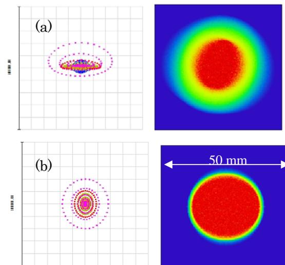
Fig.2 Spot diagrams and images of optical fiber (0.2 mm dia.) at divertor region. (a) light starts from the edge of the fiber array (b) light starts from the center of the fiber array
