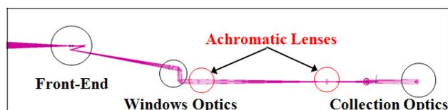
Fig. 1 Top view of the new equatorial port optics. Two achromatic lenses are installed outside the vacuum vessel.
