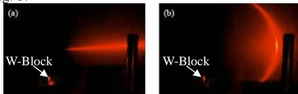
Fig.3 Image of the reflected light (a) light incident perpendicular to engraved lines (b) light incident parallel to the engraved lines
