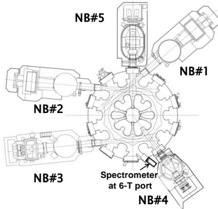
Fig. 2. Arrangement of neutral beam injectors in LHD and a position of the spectrometer in this calculation.
