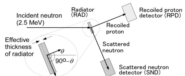
Fig. 1. Schematic diagram of the associated particle coincident counting – neutron spectrometer.
