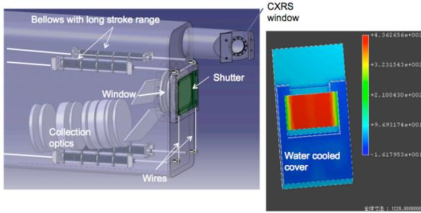
Fig. 2 Design of shutter in the P2 horizontal port plug for Thomson scattering measurement.
