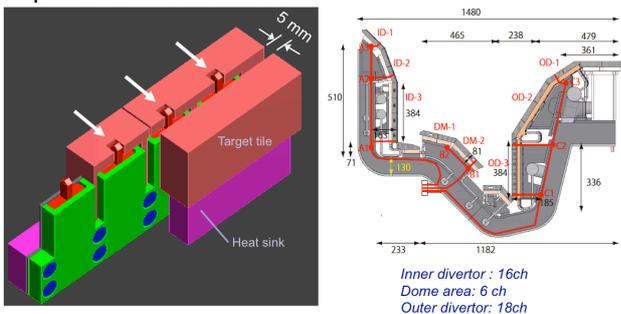
Fig. 3 Langmuir probes installed in the divertor target. Arrow shows direction of the plasma flow.
