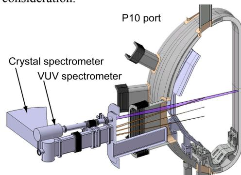
Fig. 4 Viewing chords of the VUV and crystal spectrometers
