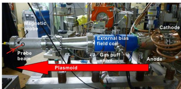
Figure 1: A picture of the developed plasma gun device in Nagoya University.
