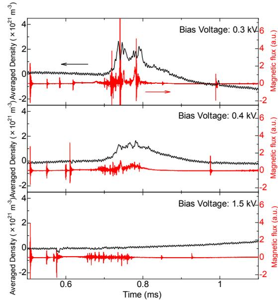
Figure 4: The temporal evolution of the electron density measure with interferometer and the signal of a magnetic probe.
