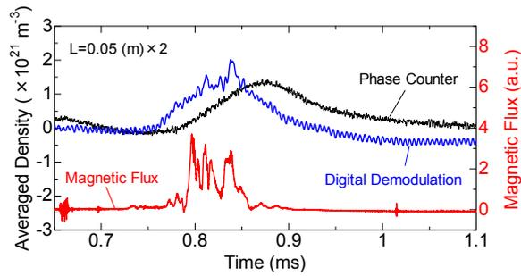
Figure 3: The temporal evolutions of the electron density measured with interferometer and the signal of a magnetic probe. The density is evaluated two methods: the analog phase counter and the digital demodulation technique.
