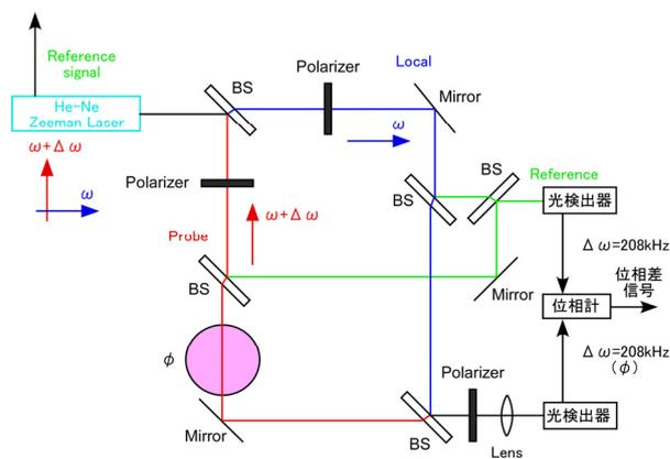
Figure 2: A schematic of the optical system of the He-Ne Zeeman laser interferometer.
