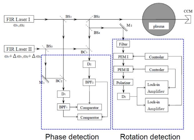
Fig.1. Schematic drawing of a combined system of the two color laser interferometer/polarimeter.
