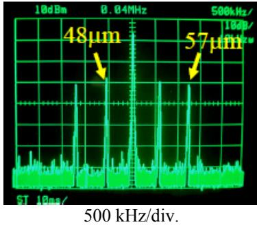
Fig. 2 Two color beat signals detected by the Ge:Ga photoconductor. The spectrum analyser trace shows two color beat signals corresponding to a  $57.2 \mu\text{m}$  beat of  $1.2 \text{ MHz}$  and a  $47.6 \mu\text{m}$  beat of  $0.55 \text{ MHz}$ .
