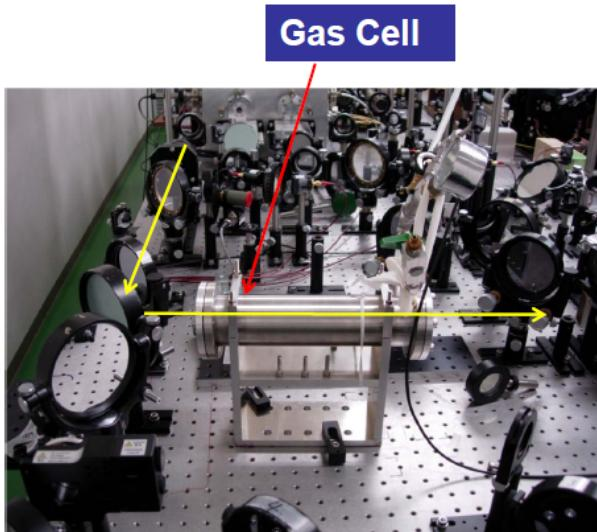
Fig. 3. A photograph of the bench testing of the two color laser interferometer/polarimeter.
