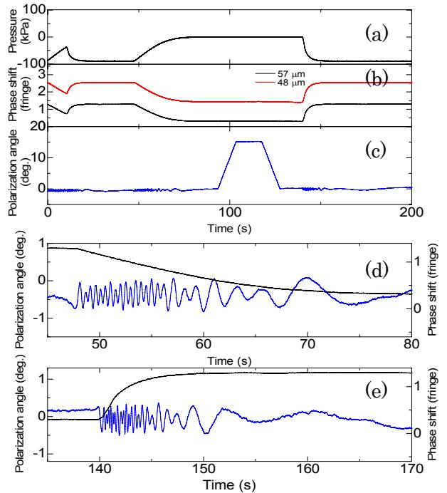
Fig. 4. Time behaviors of (a) pressure of a gas cell, (b) phase shifts of two color laser interferometers, and (c) polarization angle. (d) and (e) are expanded scale plots of the polarization angle and the phase shift.
