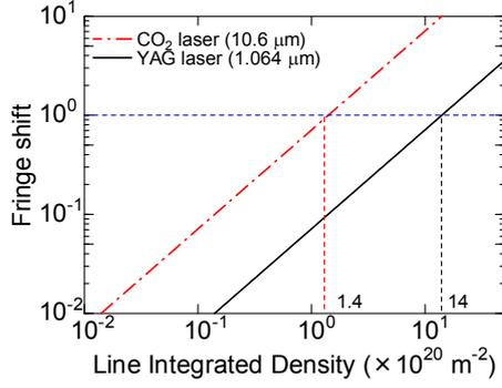
Fig. 2: Dependence of the fringe shifts of the dispersion interferometer on the laser sources.
