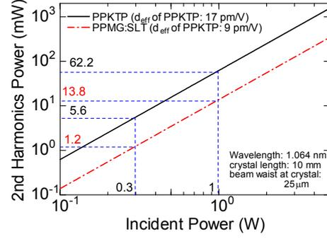
Fig. 3: Generated power of the second harmonics with PPMg:SLT and PPKTP.
