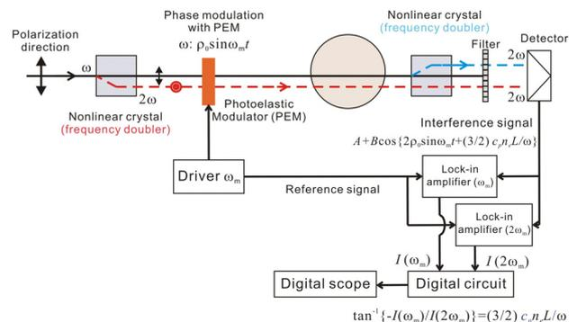
Fig. 1: Schematic view of the dispersion interferometer using a ratio of modulation amplitude
