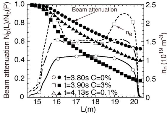
Fig. 3. Electron density and beam attenuation along the beam injection path.
