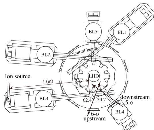
Fig. 1. Schematic drawing of neutral beam injectors and line of sights for beam attenuation measurement in LHD.
