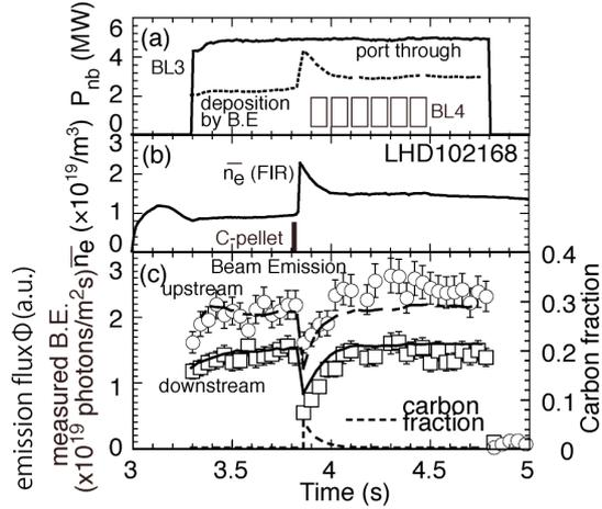
Fig. 2. (a) Bold line is the injection NB power of BL3 and dotted line is the deposition power estimated by beam attenuation analysis. (b) Line averaged electron density. (c) Beam emission intensities at the upstream and the downstream positions. Lines are beam emission flux calculated by beam attenuation analysis using ADAS database on the assumption of decaying a carbon fraction.
