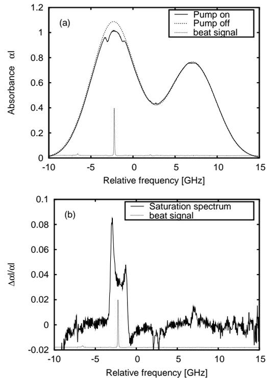
Figure 2: (a) Spectra of absorbance with and without the pump laser, and (b) spectrum of saturation spectroscopy.
