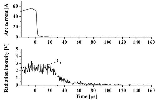
Fig. 5: Radiation intensity of  $C_2$  in PA66 ablated arc.
