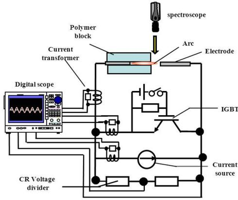
Fig. 2: Layout of experimental circuit.
