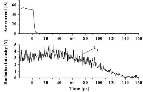
Fig. 6: Radiation intensity of  $C_2$  in PTFE ablated arc.
