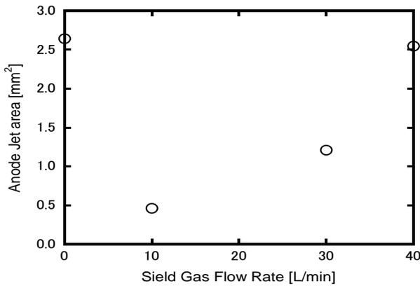
Fig.3. Effect of shield gas flow rate on anode jet area.
