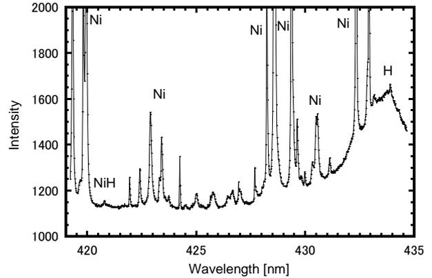
Fig.5. Emission spectrum of Ar-H<sub>2</sub> arc.
