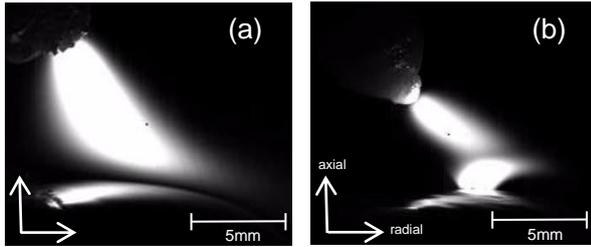
Fig.2. High-speed camera images of (a) 100%-Ar arc (b) 30%-H<sub>2</sub> arc.
