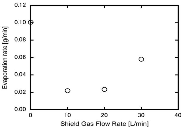
Fig.4. Effect of shield gas flow rate on evaporation rate.
