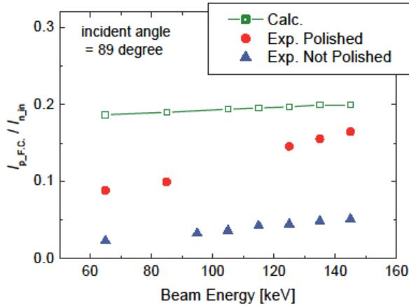
Fig. 1 The  $H^+$  beam current integrated over the beam profile divided by the initial  $H^+$  beam current, with the non-polished stripper (triangles) and with the polished stripper (circles). The squares indicate the results of TRIM calculation.
