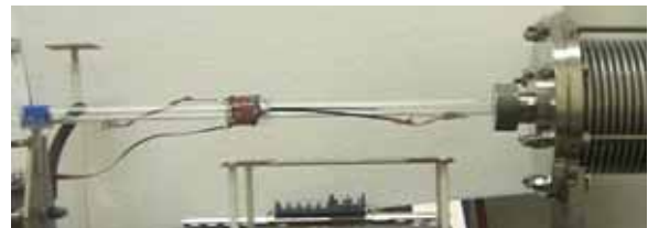
Fig.2. Photography of vacuum chamber with antenna of rotating magnetic field.
