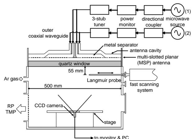
Fig.1. Experimental setup for plasma production.
