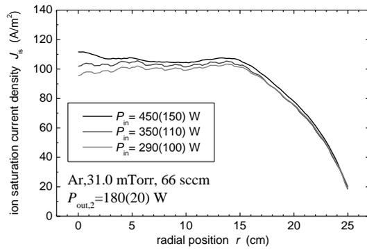
Fig.2. The dependence of radial distribution of  $J_{is}$  on  $P_{in,1}$ .
