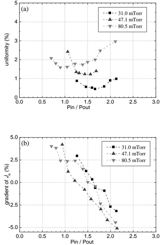
Fig.3. The dependence of the plasma parameters on the power ratio: (a) uniformity and (b) gradient.
