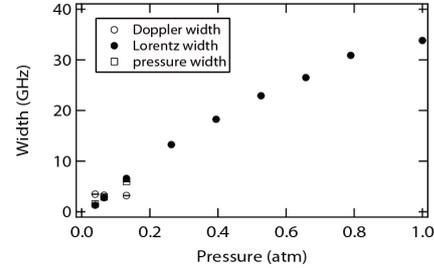
Fig. 4. Pressure dependence of the Doppler, Lorentz and pressure widths.
