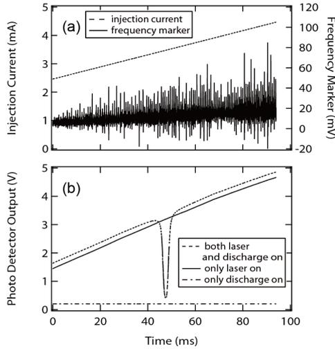
Fig. 2. An example of raw data. (a) The injection current to the laser diode and the frequency marker signal. (b) The photo-detector signals.
