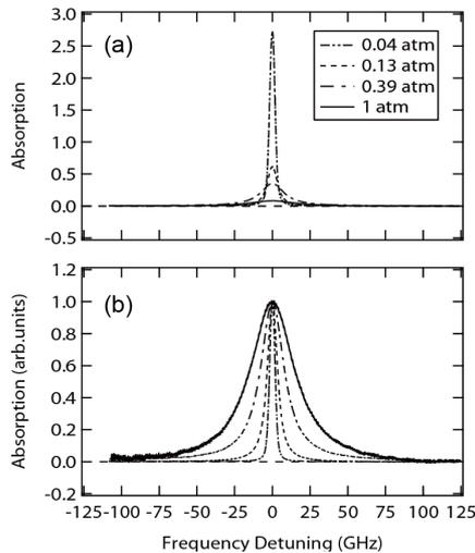
Fig. 3. (a) Absorption spectra at gas pressures at 0.04, 0.13, 0.40, 1 atm. (b) Normalized absorption spectra.
