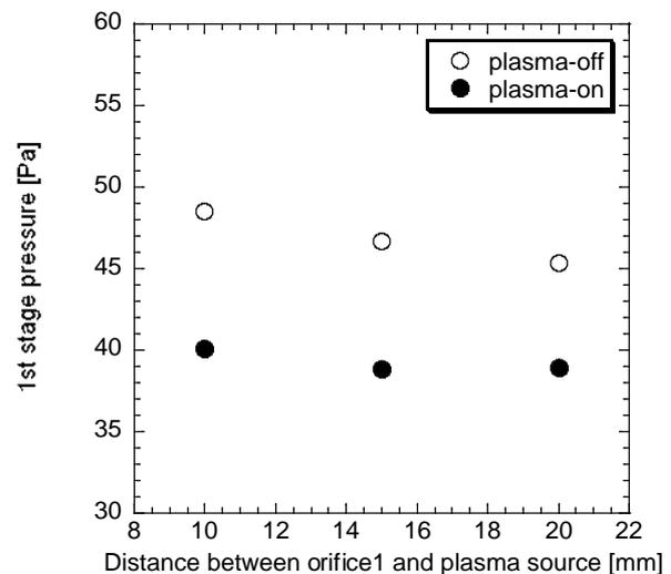
Fig.5. Dependency of 1st stage pressure on the distance between the nozzle of plasma device and orifice 1 with or without helium plasma jet.
