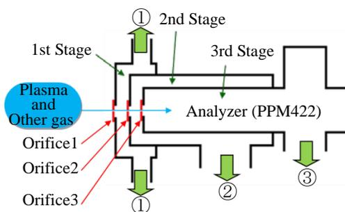
Fig.2. Differential pumping system.
