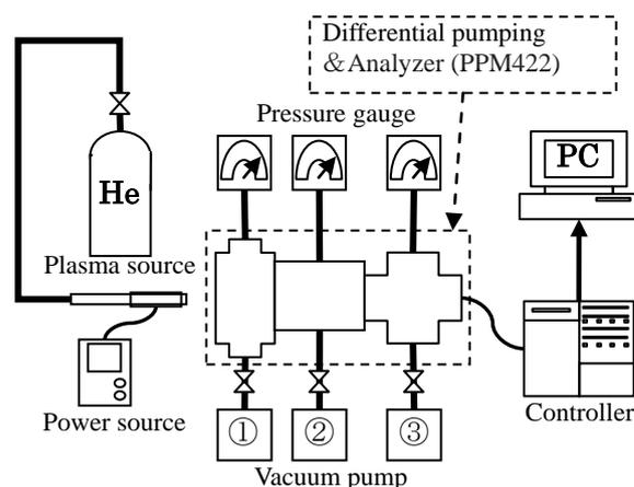
Fig.1. Mass spectrometry system.
