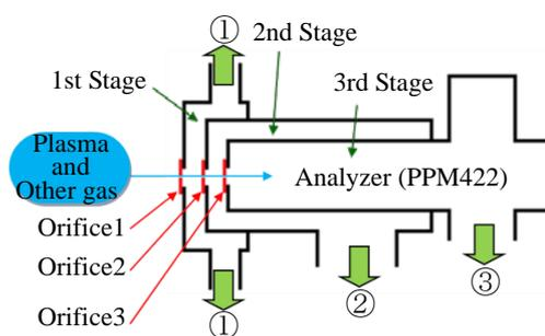
Fig.2. Differential pumping system.
