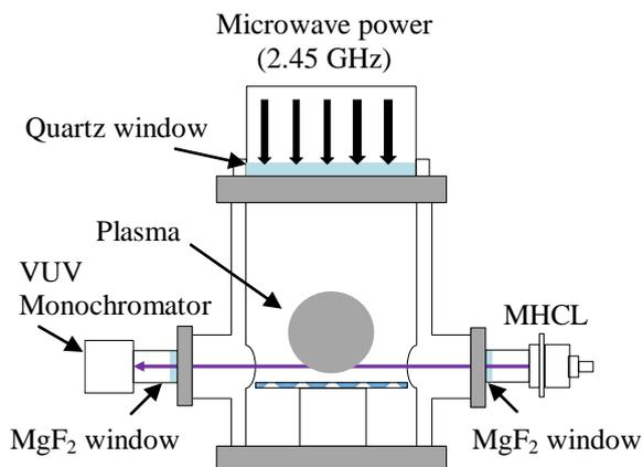
Fig. 1 Schematic of experimental set-up used for C atom density measurement with MHCL (micro-discharge hollow-cathode lamp) as a VUV light source.
