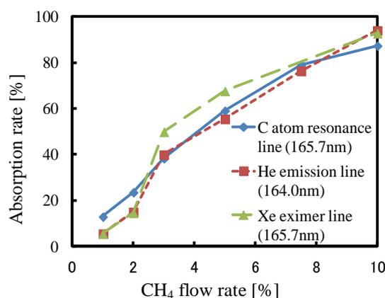
Fig. 2 Absorption rate of C atom line and background absorption as a function of CH<sub>4</sub> flow rate
