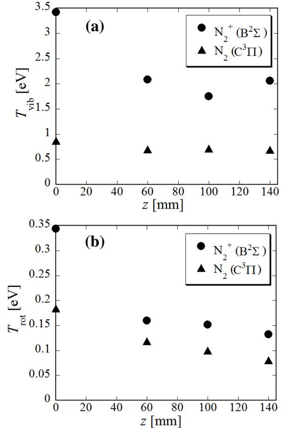
Fig.3. Vibrational and rotational temperatures measured experimentally (a) vibrational temperature of  $N_2$  ( $C^3\Pi$ ) and  $N_2^+$  ( $B^2\Sigma$ ) (b) rotational temperature of  $N_2$  ( $C^3\Pi$ ) and  $N_2^+$  ( $B^2\Sigma$ ).
