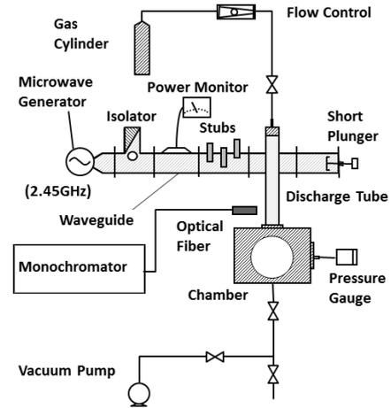
Fig.1. Block diagram of microwave discharge apparatus and measurement system
