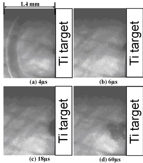
Fig. 3 Shadow graph images of the ablation space in supercritical water (30 MPa and 430°C) at various delay times after laser ablation..
