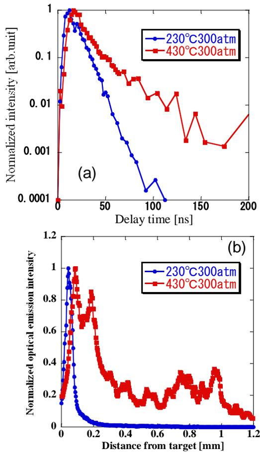
Fig. 2 (a) Temporal variations and (b) spatial distributions of optical emission intensities from laser ablation plasmas produced in liquid water (30 MPa, 230°C) and supercritical water (30 MPa, 430°C).
