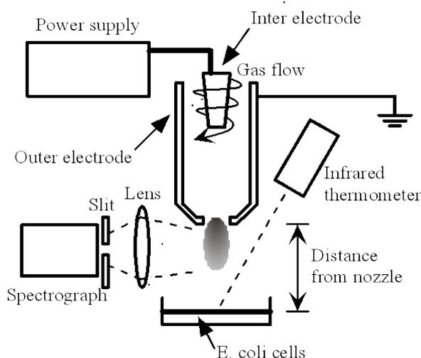
Fig.1. Schematic of the germicidal treatment by plasma jet, spectroscopic measurement, and thermometry.
