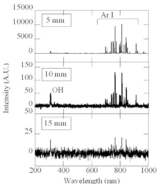
Fig. 2 UV/visible emission spectra of Ar plasma jet sources in the wavelength range from 250 to 1000 nm, where distance from nozzle
