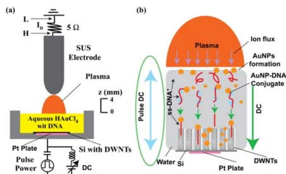
Fig. 1. (a) Schematic of the experimental setup, and (b) mechanism of the synthesis of AuNP-DNA conjugate decorated DWNTs.
