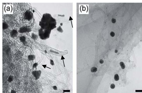
Fig. 2. TEM images of samples with superimposed DC voltage of (a) +200 V and (b) -200 V. Scale bar is 20 nm.
