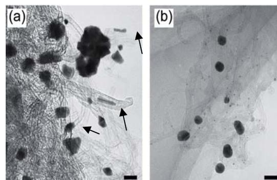
Fig. 2. TEM images of samples with superimposed DC voltage of (a) +200 V and (b) -200 V. Scale bar is 20 nm.
