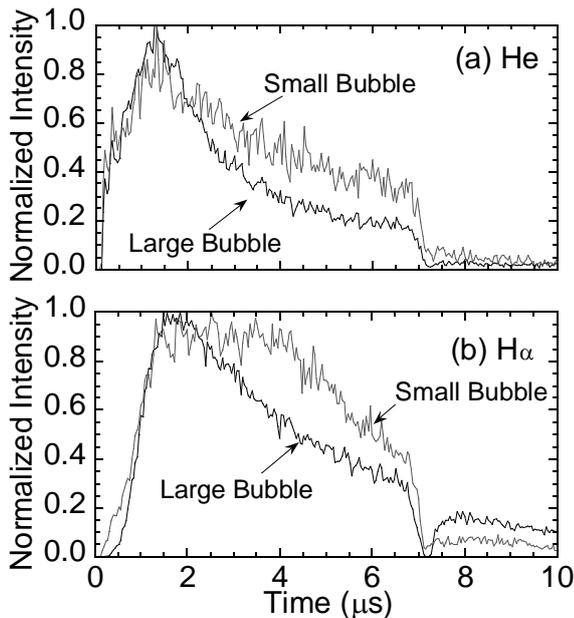
Fig. 3. Temporal variation of (a) He I and (b)  $H_\alpha$  emission from the plasma for the cases of small and large bubbles.
