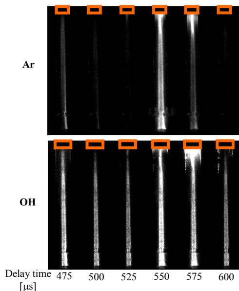
Fig. 2 The comparison of the emission from Ar and OH radicals
