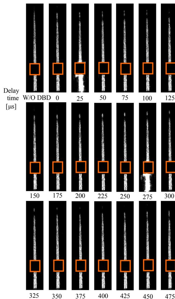
Fig. 3 The change in the flame shape and the emission intensity from OH
