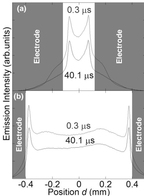
Fig. 2. Optical emission profiles of (a)  $d=0.2$  mm and (b)  $d=0.8$  mm.
