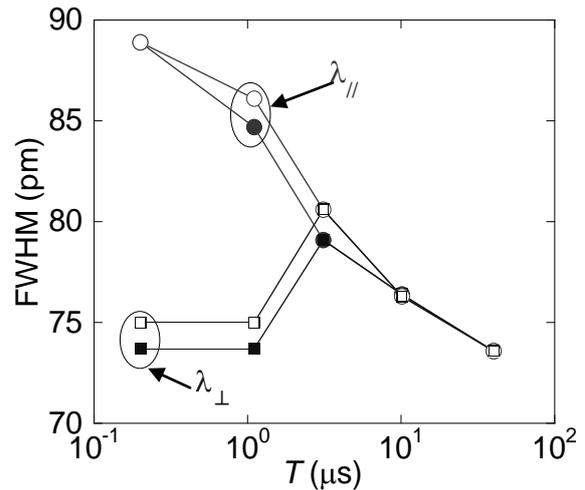
Fig. 3.  $\Delta\lambda_{//}$  and  $\Delta\lambda_{\perp}$ , as a function of  $T$ . Open and closed symbols denote measurements in the vicinities of lower and upper slot electrodes, respectively. Slot width is 0.8 mm.
