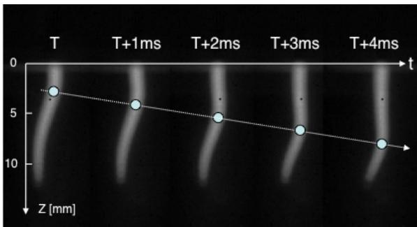
Fig. 2. Propagation of a flame structure of the plasma torch (Ar: 4 L/min, Microwave power: 100W).
