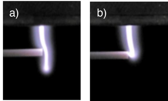
Fig. 4. Comparison of the influence of probe electrodes on the structure of plasma; (a) insulator, (b) metal electrode (single probe)
