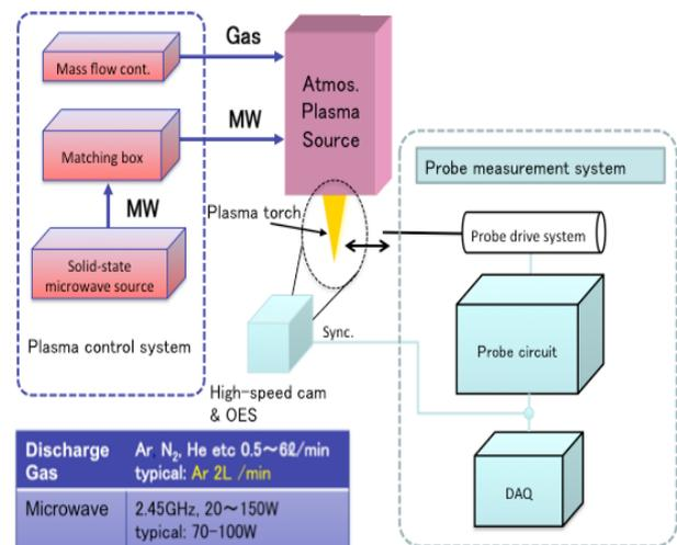
Fig. 1. Experimental setup for observing an atmospheric pressure microwave plasma torch using a high-speed camera and an electrical probe.
