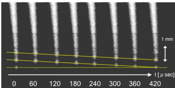
Fig. 3. Observation of a fragmental structure at the tip of the plasma torch (Ar: 4 L/min, Microwave power: 100W).
