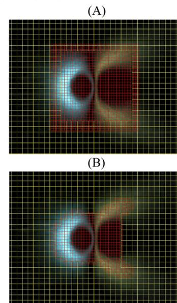
Fig.1. Grid arrangement and current density profile resulting from AMR simulations in two different refinement criteria. Red and yellow lattices represent refined and coarse grid regions, respectively.
