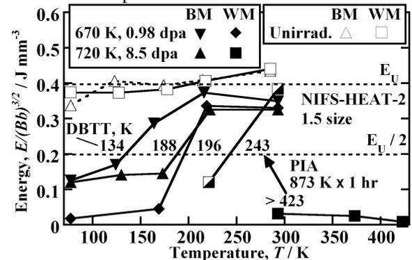
Fig. 2 Absorbed energy for Charpy impact tests with 1/3 size specimens.
