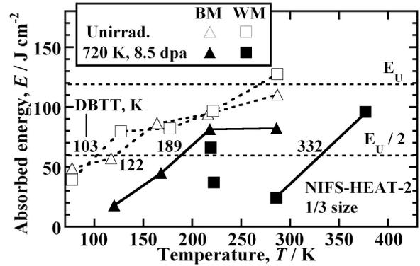
Fig. 1 Absorbed energy for Charpy impact tests with 1/3 size specimens.
