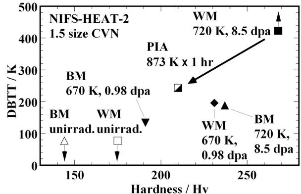
Fig. 3 Relationship between DBTT and hardness of the base metal and the weld metal before and after the neutron irradiations.
