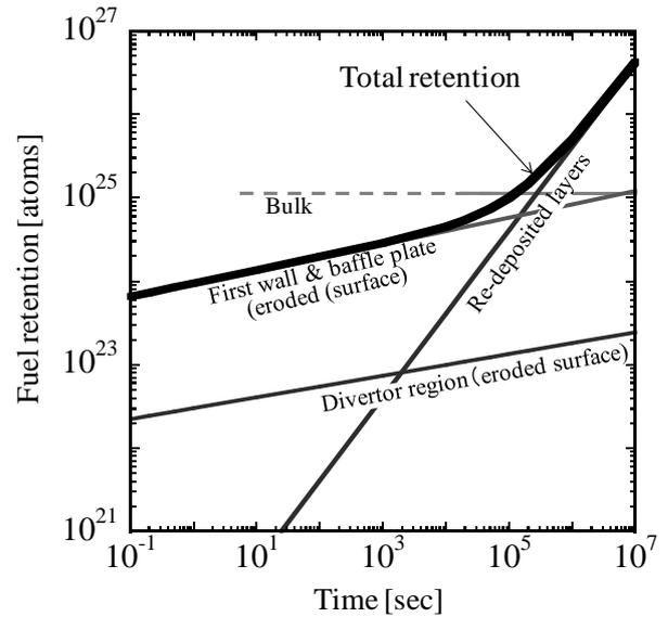
Fig.1. Fuel retention build-up in JT-60U according to the present modeling with four different mechanisms for retentions in re-deposited layers, two different eroded surfaces and bulk. Note that T inventory limit of ITER (700 g T) is  $1.4 \times 10^{26}$  atoms.
