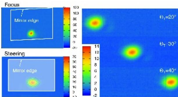
Fig. 3. Measured field pattern of radiated beam at the surface of M1 and M2 and the outlet of the EL mock-up.
