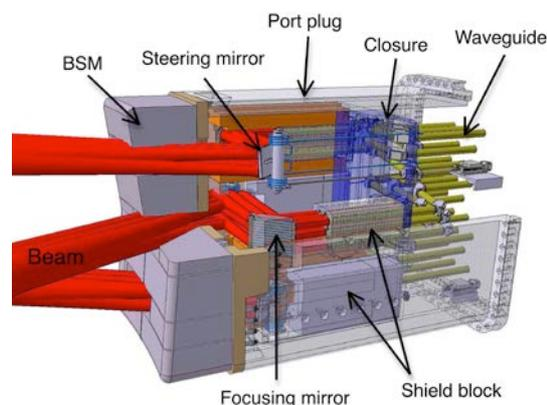
Fig. 2. Present design of ITER equatorial EC launcher : The 20MW power is provided by three beam bundles and one of them is injected for the evolution of counter current drive.
