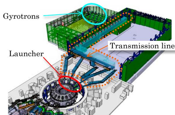
Fig. 1. ITER EC H&CD system : Gyrotrons and transmission line and launchers.
