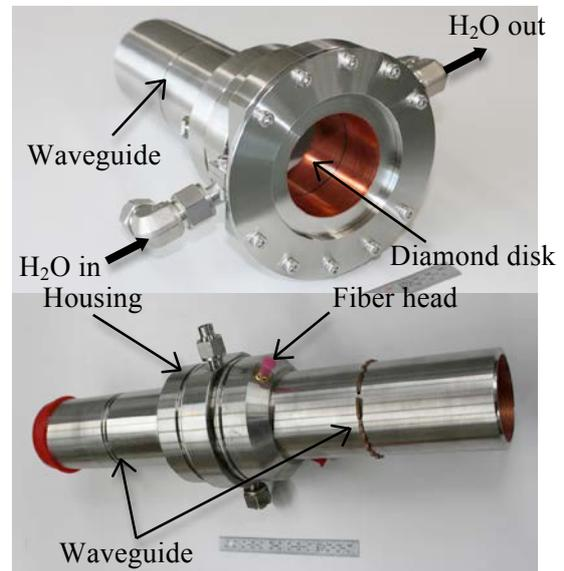
Fig. 4. Photograph of a torus diamond window prototype for ITER EC H&CD system.
