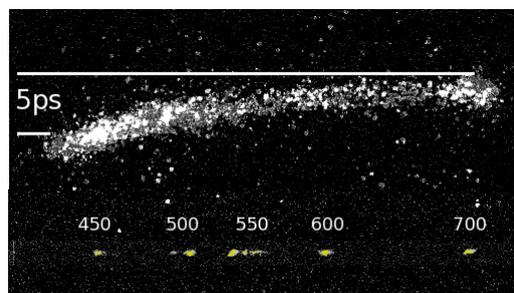
Fig.1 White pulse profile by streak camera
