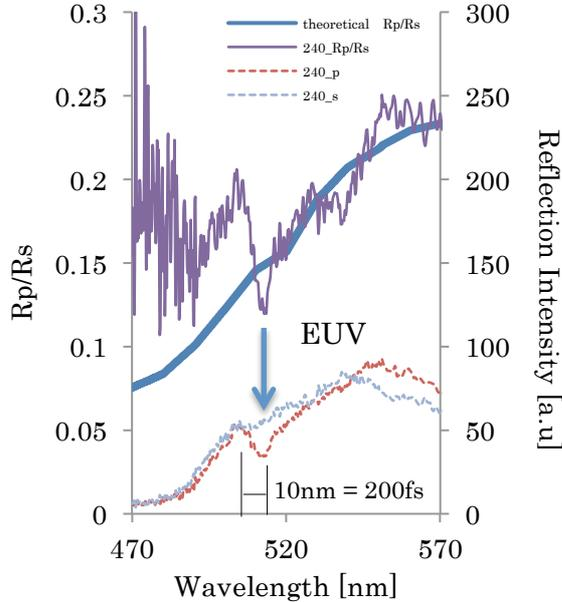
Fig. 3 Au 10.2 nm film target reflection intensity changed by EUV-FEL. Blue line is Calculate Rp/Rs. Purple line is actual measured Rs/Rp. Red dashed line is reflection intensity of p polarization. Red dash-dot line is reflection intensity of s polarization.
