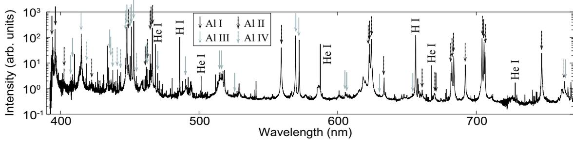
Fig. 2. Emission spectrum of an aluminum pellet ablation cloud in LHD. The relative intensity is calibrated.
