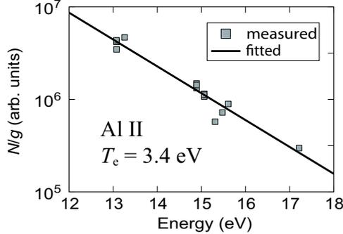
Fig. 3. Populations of  $\text{Al}^+$  excited levels per unit statistical weight as a function of the excitation energy.
