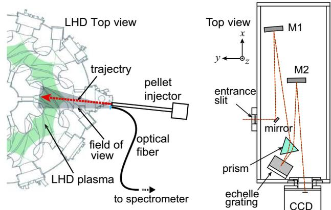
Fig. 1. A schematic illustration of the experimental set-up (left) and the echelle spectrometer (right).
