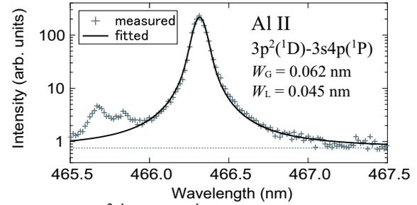
Fig. 4. Al II  $3p^2(^1D)-3s4p(^1P)$  emission line profile. The solid line is the result of Voigt function fit. The dotted line indicates the background signal level for the fit.
