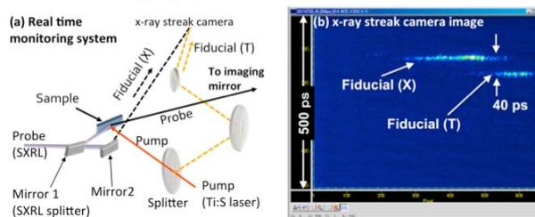
Fig.3. Real time pulse monitoring system for the temporal adjustment between pump and probe pulses.
