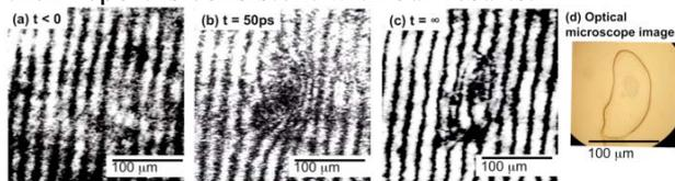
Fig.2. Temporal evolution of the interferogram and optical microscope image of the laser induced Pt surface.
