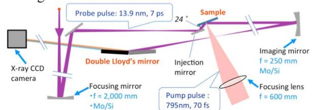
Fig.1. Single shot pump & probe interferometer.
