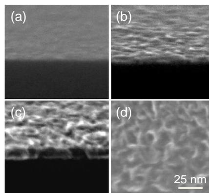
Fig.1 SEM images of initial growth surfaces of CNW: birds-eye view images at (a) 2min (b) 5 min and (c) 22 min, and (d) top-view image at 22 min.
