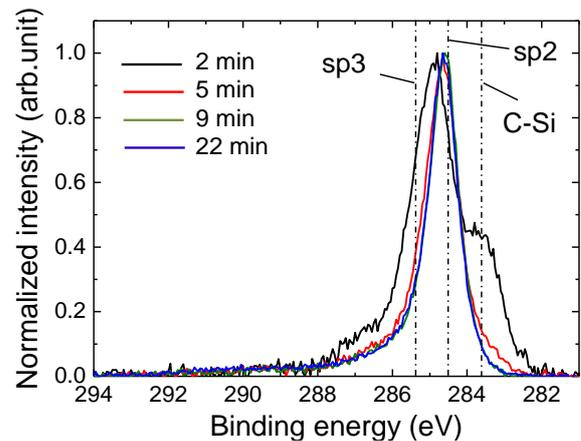
Fig.3 C 1s spectra of initial layer of CNWs at growth time of 2 to 22 min.
