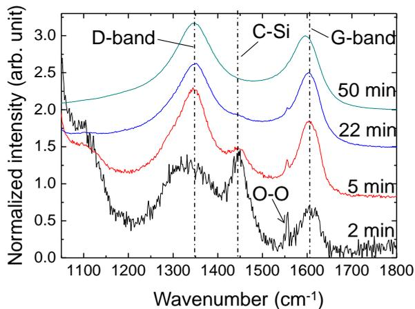
Fig.2 Raman spectra of initial layer of CNWs
